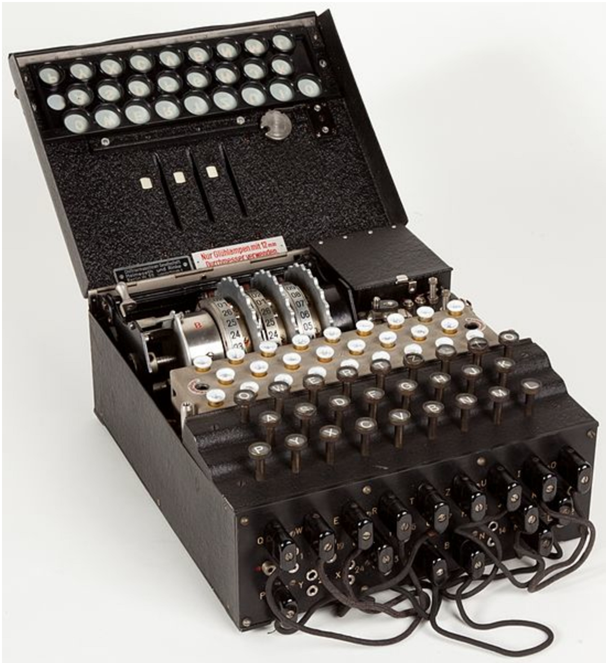
Fig. 1: Military Enigma machine, model “Enigma 1”, used during the late 1930s and during the war (from https://brilliant.org/wiki/enigma-machine/ )
